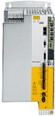
Drive-based motion control system With expansion card PMCprimo C Standard bus system: CANopen Software option: IEC 61131-3 programming Technical data at 3 x 400 V AC: Continuous output current: 48 A, Imax (5 s)= 96 A, power consumption in S1 operation: 35 kVA required accessories: Brake resistor 15 Ohm.
