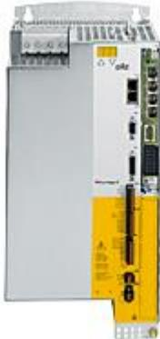
Included extension board PMCprimo C Bussystems standard: CANopen / Profibus-DP-S Software option: IEC61131-3 programming yy Technical Details at 3 x 400 V AC supply voltage: Permanent output current: 48 A; Imax (5 sec.) = 96 A; Power consumption in S1 operation: 35 kVA necessary accessories: brake resistor 15 OHM
