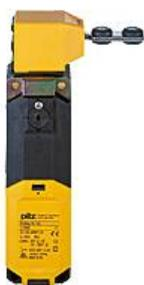
Mechanical safety switch with standard actuator Interlock principle: Spring force 1500 N; contacts: 2 N/O, 2 N/C Supply voltage 110V - 230 V AC.
