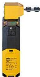
Mechanical safety switch with standard actuator Interlock principle magnetic force Contacts 2 N/O, 2 N/C Supply voltage 24 V AC/DC.
