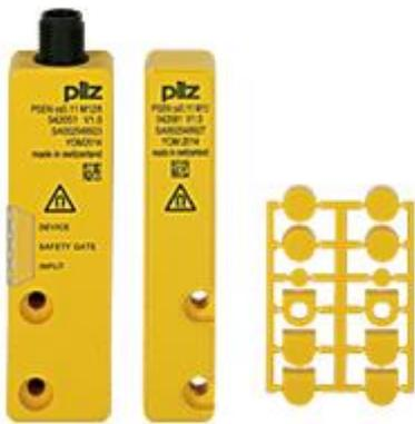
RFiD safety switch 2 safe semiconductor outputs, 8-pin M12 connector, IP67, 4 directions of actuation, Operating distance (direction of actuation square): 11 mm, Sao = 8 mm, Sar = 20 mm, PU = 1 piece coded switch with actuator, magnetic latching.
