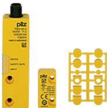
RFid safety switch 2 safe semiconductor outputs, 8-pin M8 connector, IP67, 4 directions of actuation, Operating distance (direction of actuation square): 11 mm, Sao = 8 mm, Sar = 20 mm, PU = 1 piece unique, fully coded switch with actuator.
