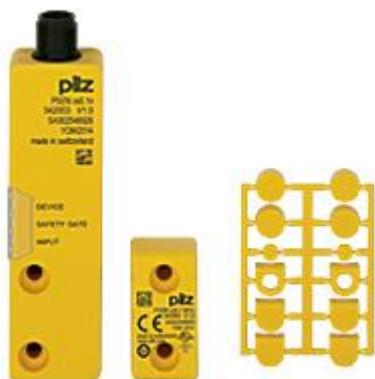
RFID safety switch 2 safe semiconductor outputs, 5-pin M12 connector, IP67, 4 directions of actuation, Operating distance (direction of actuation square): 11 mm, Sao = 8 mm, Sar = 20 mm, PU = 1 piece fully coded switch with actuator A total of 8 learning procedures are possible.
