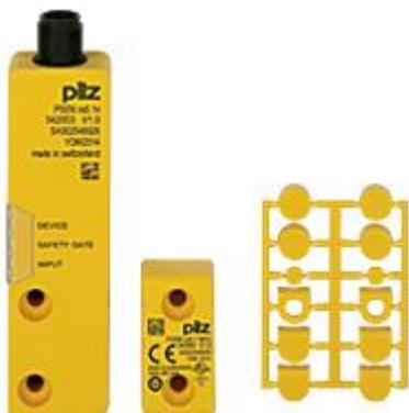
RFID safety switch 2 safe semiconductor outputs, 8-pin M12 connector IP67, 4 directions of actuation, Operating distance (direction of actuation square): 11 mm, Sao = 8 mm, Sar = 20 mm, PU = 1 piece coded switch with actuator.
