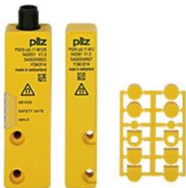
Non-contact coded safety switch for position monitoring of movable guards according to EN 60947-5-3; two safe outputs; connector M12/5pin. For applications up to SILCL 3 resp PLe; IP 67, typical switching distance (rectangle) 11mm,  $S_{ao}=8\text{mm}$ ,  $S_{ar}=20\text{mm}$ ; packaging unit = 1 piece fully coded switch and 1 piece actuator: Teach-in of 8 other actuators possible; Magnetic latching
