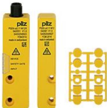
Non-contact coded safety switch for position monitoring of movable guards according to EN 60947-5-3; two safe outputs; connector M12/5pin. For applications up to SILCL 3 resp PLe; IP 67, typical switching distance (rectangle) 11mm,  $S_{ao}=8\text{mm}$ ,  $S_{ar}=20\text{mm}$ ; packaging unit = 1 piece unique coded switch and 1 piece actuator: Teach-in of other actuators not possible; magnetic latching
