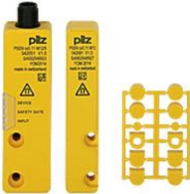
RFid safety switch 2 safe semiconductor outputs, 8-pin M12 connector, IP67, 4 directions of actuation, Operating distance (direction of actuation square): 11 mm, Sao = 8 mm, Sar = 20 mm, PU = 1 piece fully coded switch with actuator A total of 8 learning procedures are possible; , magnetic latching.
