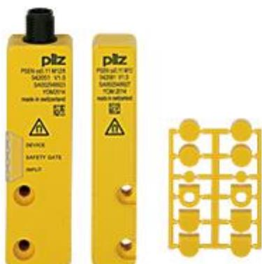
Non-contact coded safety switch for position monitoring of movable guards according to EN 60947-5-3; two safe outputs; connector M12/5pin. For applications up to SILCL 3 resp PLe ; IP 67, typical switching distance 11mm, Sao=8mm, Sar=20mm packaging unit = 1piece fully coded switch with 1 piece actuator; Teach-in of other actuators not possible.
