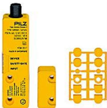
RFid safety switch 2 safe semiconductor outputs, 8-pin M12 connector, IP67, 4 directions of actuation, Operating distance (direction of actuation square): 11 mm, Sao = 8 mm, Sar = 20 mm, PU = 1 piece coded switch with actuator, ATEX approval.
