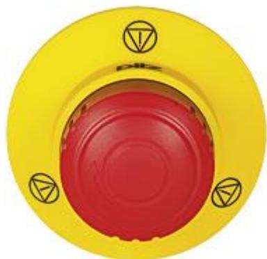
PITestop E-STOP pushbutton IP65, large with E-STOP symbol and with logo, mounting hole: 22.3 mm.
