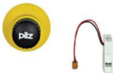
PITestop operating stop pushbutton IP65, LED ring illumination incl. connection module Mounting hole: 22.3 mm.
