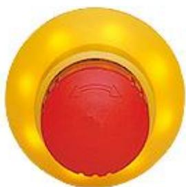
PITestop E-STOP pushbutton IP65, illuminated, without logo, mounting hole: 22.3 mm.
