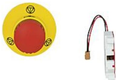
PITestop E-STOP pushbutton IP65, illuminated with E-STOP symbol and with logo and spring-loaded terminals, mounting hole: 22.3 mm.
