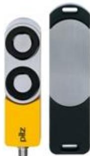
Magnetic safety gate system For applications up to SIL 3/PL e/cat. 4 magnetic holding force 1000 N (process protection). Coding: uniquely, fully coded; 8-pin M12 connector male; 4 LEDs Delivery scope: 1 sensor with free-moving actuator.
