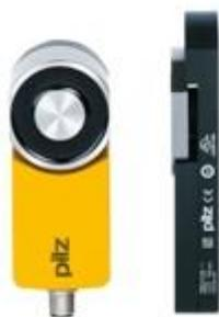
Safety gate system with magnetic interlock, IP67, 8pin M12 connector (male). 2 safe semiconductor outputs (OSSD); Solenoid power 500N (process guarding); 4 LEDs; Applications up to SIL3/PL e/Cat4; additional function: safe semiconductor outputs are high if door is closed (independent from guardlocking function); Content = 1 fully coded Sensor with free-moving actuator. Teach-in of new actuators up to 8 times."
