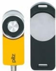
Magnetic safety gate system For applications up to SIL 3/PL e/cat. 4 magnetic holding force 500 N (process protection). Coding: fully coded; 5-pin M12 male connector; 4 LEDs.
