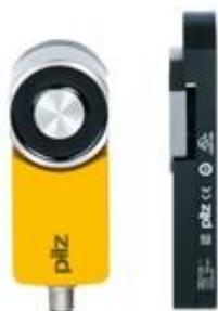
Safety gate system with magnetic interlock, IP67, 8pin M12 connector (male). 2 safe semiconductor outputs (OSSD); Solenoid power 500N (process guarding); 4 LEDs; Applications up to SIL3/PL e/Cat4; additional function: safe semiconductor outputs are high if door is closed (independent from guardlocking function); Content = 1 coded Sensor with free-moving actuator."
