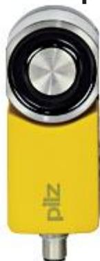
Safety gate system with magnetic interlock, IP67, 8pin M12 connector (male). 2 safe semiconductor outputs (OSSD); Solenoid power 500N (process guarding); 4 LEDs; Applications up to SIL3/PL e/Cat4; additional function: Extended diagnostics for serial connection; Content = 1 fully coded Sensor without actuator. Teach-in of new actuators up to 8 times.
