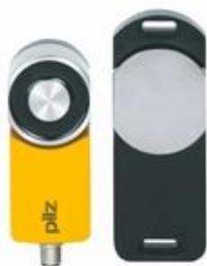
Safety gate system with magnetic interlock, IP67, 5pin M12 connector (male). 2 safe semiconductor outputs (OSSD); Solenoid power 500N (process guarding); 4 LEDs; Applications up to SIL3/PL e/Cat4; additional function: safe semiconductor outputs are high if door is closed (independent from guardlocking function); Content = 1 unique fully coded Sensor with actuator. No teach-in of new actuators."
