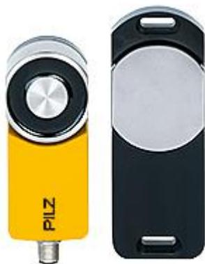
Magnetic safety gate system For applications up to SIL 3/PL e/cat. 4 magnetic holding force 500 N (process protection). Coding: coded; 5-pin M12 male connector; 4 LEDs.
