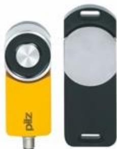
Magnetic safety gate system For applications up to SIL 3/PL e/cat. 4 magnetic holding force 500 N (process protection). Coding: fully coded; 8-pin M12 male connector; 4 LEDs.
