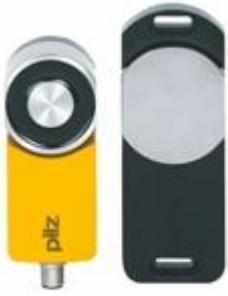
Safety gate system with magnetic interlock, IP67, 5pin M12 connector (male). 2 safe semiconductor outputs (OSSD); Solenoid power 500N (process guarding); 4 LEDs; Applications up to SIL3/PL e/Cat4; additional function: Extended diagnostics for serial connection; Content = 1 fully coded Sensor with actuator. Teach-in of new actuators up to 8 times"
