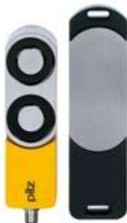
Magnetic safety gate system For applications up to SIL 3/PL e/cat. 4 magnetic holding force 1000 N (process protection). Coding: coded; 5-pin M12 connector male; 4 LEDs Delivery scope: 1 sensor with free-moving actuator.
