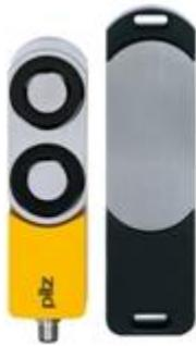
Safety gate system with magnetic interlock, IP67, 8pin M12 connector (male). 2 safe semiconductor outputs (OSSD); Solenoid power 1000N (process guarding); 4 LEDs; Applications up to SIL3/PL e/Cat4; additional function: Extended diagnostics for serial connection; Content = 1 piece fully coded and free-moving actuator. Teach-in of new actuators up to 8 times."
