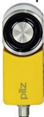
Magnetic safety gate system For applications up to SIL 3/PL e/cat. 4 magnetic holding force 500 N (process protection). Coding: coded; 8-pin M12 male connector; 4 LEDs.
