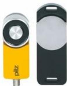
Safety gate system with magnetic interlock, IP67, 5pin M12 connector (male). 2 safe semiconductor outputs (OSSD); Solenoid power 500N (process guarding); 4 LEDs; Applications up to SIL3/PL e/Cat4; additional function: safe semiconductor outputs are high if door is closed (independent from guardlocking function); Content = 1 fully coded Sensor with actuator. Teach-in of new actuators up to 8 times"
