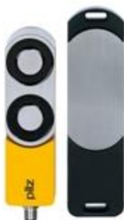
Safety gate system with magnetic interlock, IP67; 8pin M12 connector (male); 2 safe semiconductor outputs (OSSD); Solenoid power 1000N (process guarding); 4 LEDs; Applications up to SIL3/PL e/Cat4; additional function: safe semiconductor outputs are high if door is closed (independent from guardlocking function); Content = 1 coded and actuator."
