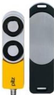
Magnetic safety gate system For applications up to SIL 3/PL e/cat. 4 magnetic holding force 1000 N (process protection). Coding: fully coded; 8-pin M12 connector male; 4 LEDs Delivery scope: 1 sensor with free-moving actuator.
