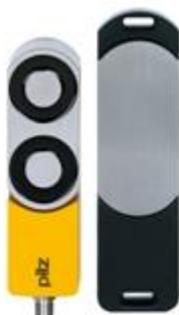
Magnetic safety gate system For applications up to SIL 3/PL e/cat. 4 magnetic holding force 1000 N (process protection). Coding: coded; 8-pin M12 connector male; 4 LEDs. Delivery scope: 1 sensor with free-moving actuator.
