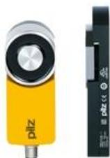
Magnetic safety gate system For applications up to SIL 3/PL e/cat. 4 magnetic holding force 500 N (process protection). Coding: fully coded; 8-pin M12 male connector; 4 LEDs.
