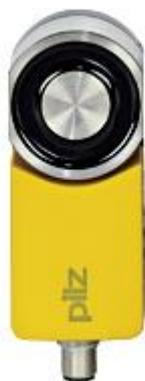
Safety gate system with magnetic interlock, IP67, 8pin M12 connector (male). 2 safe semiconductor outputs (OSSD); Solenoid power 500N (process guarding); 4 LEDs; Applications up to SIL3/PL e/Cat4; additional function: safe semiconductor outputs are high if door is closed (independent from guardlocking function); Content = 1 fully coded Sensor without actuator. Teach-in of new actuators up to 8 times.
