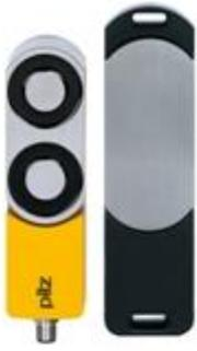
Magnetic safety gate system For applications up to SIL 3/PL e/cat. 4 magnetic holding force 1000 N (process protection). Coding: uniquely coded ; 5-pin M12 male connector; 4 LEDs. Delivery scope: 1 sensor with actuator.
