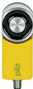
Magnetic safety gate system For applications up to SIL 3/PL e/cat. 4 magnetic holding force 500 N (process protection). Coding: fully coded; 8-pin M12 male connector; 4 LEDs.
