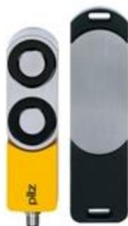
Safety gate system with magnetic interlock, IP67, 8pin M12 connector (male). 2 safe semiconductor outputs (OSSD); Solenoid power 1000N (process guarding); 4 LEDs; Applications up to SIL3/PL e/Cat4; additional function: safe semiconductor outputs are high if door is closed (independent from guardlocking function); Content = 1 piece fully coded and free-moving actuator. Teach-in of new actuators up to 8 times."
