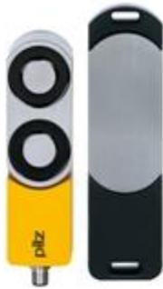
Safety gate system with magnetic interlock, IP67; 2 safe semiconductor outputs (OSSD); Solenoid power 1000N (process guarding); 4 LEDs; Applications up to SIL3/PL e/Cat4; additional function: Extended diagnostics for serial connection; Content = 1 fully coded and actuator. Teach-in of new actuators up to 8 times."
