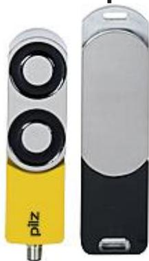
Magnetic safety gate system For applications up to SIL 3/PL e/cat. 4 magnetic holding force 1000 N (process protection). Coding: coded; 8-pin M12 male connector; 4 LEDs. Special version: Base plates from stainless steel (1.4301) + stainless steel connector Delivery scope: 1 sensor with free-moving actuator.
