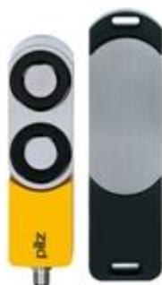
Magnetic safety gate system For applications up to SIL 3/PL e/cat. 4 magnetic holding force 1000 N (process protection). Coding: fully coded; 5-pin M12 male connector; 4 LEDs. Delivery scope: 1 sensor with actuator.
