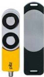
Magnetic safety gate system For applications up to SIL 3/PL e/cat. 4 magnetic holding force 1000 N (process protection). Coding: uniquely, fully coded; 5-pin M12 connector male; 4 LEDs Delivery scope: 1 sensor with free-moving actuator.
