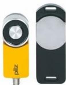
Magnetic safety gate system For applications up to SIL 3/PL e/cat. 4 magnetic holding force 500 N (process protection). Coding: uniquely coded ; 5-pin M12 male connector; 4 LEDs.
