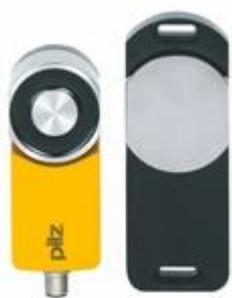
Magnetic safety gate system For applications up to SIL 3/PL e/cat. 4 magnetic holding force 500 N (process protection). Coding: uniquely coded ; 8-pin M12 male connector; 4 LEDs.
