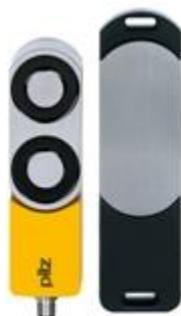
Safety gate system with magnetic interlock, IP67, 8pin M12 connector (male). 2 safe semiconductor outputs (OSSD); Solenoid power 1000N (process guarding); 4 LEDs; Applications up to SIL3/PL e/Cat4; additional function: safe semiconductor outputs are high if door is closed (independent from guardlocking function); Content = 1 piece coded and free-moving actuator."
