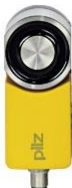
Safety gate system with magnetic interlock, IP67, 8pin M12 connector (male). 2 safe semiconductor outputs (OSSD); Solenoid power 500N (process guarding); 4 LEDs; Applications up to SIL3/PL e/Cat4; additional function: safe semiconductor outputs are high if door is closed (independent from guardlocking function); Content = 1 coded Sensor without actuator.
