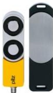
Magnetic safety gate system For applications up to SIL 3/PL e/cat. 4 magnetic holding force 1000 N (process protection). Coding: fully coded; 8-pin M12 male connector; 4 LEDs. Delivery scope: 1 sensor with actuator.
