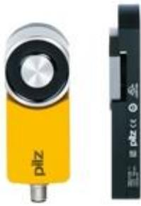
Safety gate system with magnetic interlock, IP67, 8pin M12 connector (male). 2 safe semiconductor outputs (OSSD); Solenoid power 500N (process guarding); 4 LEDs; Applications up to SIL3/PL e/Cat4; additional function: Extended diagnostics for serial connection; Content = 1 fully coded Sensor with free-moving actuator. Teach-in of new actuators up to 8 times."
