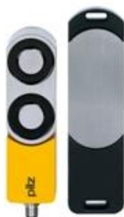
Safety gate system with magnetic interlock, IP67; 8pin M12 connector (male); 2 safe semiconductor outputs (OSSD); Solenoid power 1000N (process guarding); 4 LEDs; Applications up to SIL3/PL e/Cat4; additional function: safe semiconductor outputs are high if door is closed (independent from guardlocking function); Content = 1 fully coded switch and actuator. Teach-in of new actuators up to 8 times."
