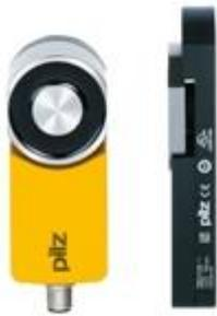
Magnetic safety gate system For applications up to SIL 3/PL e/cat. 4 magnetic holding force 500 N (process protection). Coding: uniquely coded ; 5-pin M12 male connector; 4 LEDs.
