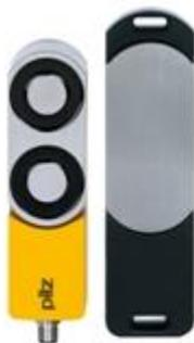
Magnetic safety gate system For applications up to SIL 3/PL e/cat. 4 magnetic holding force 1000 N (process protection). Coding: uniquely coded ; 8-pin M12 male connector; 4 LEDs. Delivery scope: 1 sensor with actuator.
