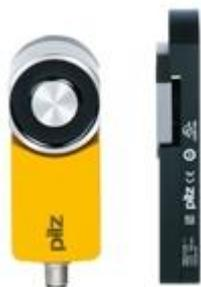
Magnetic safety gate system For applications up to SIL 3/PL e/cat. 4 magnetic holding force 500 N (process protection). Coding: coded; 8-pin M12 male connector; 4 LEDs.
