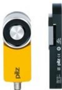
Magnetic safety gate system For applications up to SIL 3/PL e/cat. 4 magnetic holding force 500 N (process protection). Coding: uniquely coded ; 8-pin M12 male connector; 4 LEDs.
