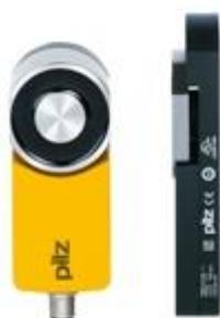
Safety gate system with magnetic interlock, IP67, 8pin M12 connector (male). 2 safe semiconductor outputs (OSSD); Solenoid power 500N (process guarding); 4 LEDs; Applications up to SIL3/PL e/Cat4; additional function: safe semiconductor outputs are high if door is closed (independent from guardlocking function); Content = 1 unique fully coded Sensor with free-moving actuator. No teach-in of new actuators."
