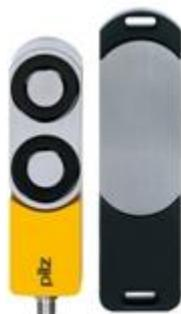
Magnetic safety gate system For applications up to SIL 3/PL e/cat. 4 magnetic holding force 1000 N (process protection). Coding: coded; 8-pin M12 male connector; 4 LEDs. Delivery scope: 1 sensor with actuator.
