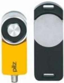
Magnetic safety gate system For applications up to SIL 3/PL e/cat. 4 magnetic holding force 500 N (process protection). Coding: coded; 8-pin M12 male connector; 4 LEDs.
