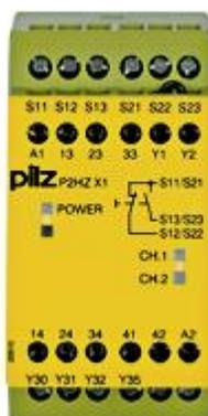
Safety relay (standalone) Inputs: 1 N/O, 1 N/C per pushbutton Outputs: 3 N/O, 1 N/C, 2 semiconductor UB 48 V AC, width: 45 mm, plug-in terminals of screw type Two-hand control device, monitoring the simultaneity of a two-hand pushbutton.
