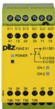
Safety relay (standalone) Inputs: 1 N/O, 1 N/C per pushbutton Outputs: 3 N/O, 1 N/C, 2 semiconductor UB 24 V DC, width: 45 mm, integral screw terminals, two-hand control device, monitoring the simultaneity of a two-hand pushbutton.
