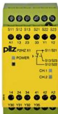
Safety relay (standalone) Inputs: 1 N/O, 1 N/C per pushbutton Outputs: 3 N/O, 1 N/C, 2 semiconductor UB 110 V AC, width: 45 mm, integral screw terminals, two-hand control device, monitoring the simultaneity of a two-hand pushbutton.
