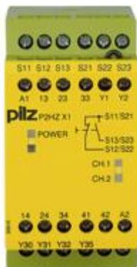
Safety relay (standalone) Inputs: 1 N/O, 1 N/C per pushbutton Outputs: 3 N/O, 1 N/C, 2 semiconductor UB 24 V AC, width: 45 mm, integral screw terminals, two-hand control device, monitoring the simultaneity of a two-hand pushbutton.
