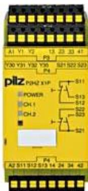
Safety relay (standalone) Inputs: 1 N/O, 1 N/C per pushbutton Outputs: 3 N/O, 1 N/C, 2 semiconductor UB 115 V AC, width: 45 mm, plug-in spring-loaded terminals. Two-hand control device/monitoring the simultaneity of two-hand pushbuttons.
