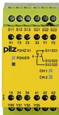
Safety relay (standalone) Inputs: 1 N/O, 1 N/C per pushbutton Outputs:3 N/O, 1 N/C, 2 semiconductor UB 230 V AC, width: 45 mm, integral screw terminals, two-hand control device, monitoring the simultaneity of a two-hand pushbutton.
