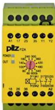
Safety relay (standalone) Inputs: Single-channel wiring Outputs: 1 N/O, 2 N/C. UB 24 V DC, width: 45 mm, integral screw terminals, delay-on energisation pulse timer, pulse times 12 stages from 0 - 600 s.
