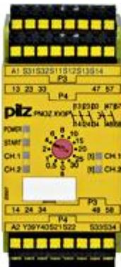
Safety relay (standalone) Inputs: 1-/2-channel wiring with/without detection of shorts across contacts Outputs: 3 N/O, 2 N/O (t = 0 - 30 s). Automatic/monitored start UB 24 V DC, width: 45 mm, plug-in spring-loaded terminals. Monitoring E-STOP, safety gates.
