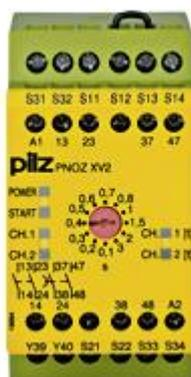
Safety relay (standalone) Inputs: 1- / 2-channel wiring with detection of shorts across contacts Outputs: 2 N/O, 2 N/O delayed UB 24 V DC, width: 45 mm, integral screw terminals, Monitoring E-STOP, safety gates with 2 delay-on de-energisation contacts. Release time 12 stages from 0 - 3 s.
