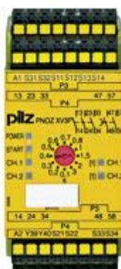
Safety relay (standalone) Inputs: 1-/2-channel wiring with/without detection of shorts across contacts Outputs: 3 N/O, 2 N/O (t = 0 - 3 s) . Automatic/monitored start UB 24 V DC, width: 45 mm, plug-in spring-loaded terminals. Monitoring E-STOP, safety gates.
