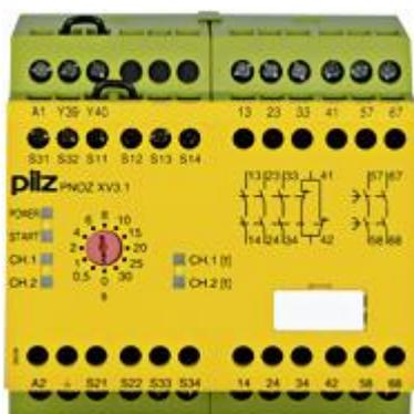
Safety relay (standalone) Inputs: 1-/2-channel wiring with/without detection of shorts across contacts Outputs: 3 N/O, 1 N/C, 2 N/O delayed UB 24-240 V AC/DC, width: 90 mm, integral screw terminals, Monitoring E-STOP, safety gates with 2 delay-on de-energisation contacts. Release time 12 stages from 0 - 30 s.
