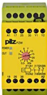
Safety relay (standalone) Inputs: Single-channel wiring Outputs: 1 N/O, 2 N/C UB 24 V DC, width: 45 mm, integral screw terminals Pulse timer, pulse times 12 stages from 0 - 30 s.
