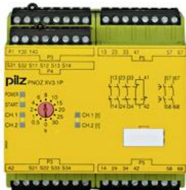
Safety relay (standalone) Inputs: 1-/2-channel wiring with/without detection of shorts across contacts Outputs: 3 N/O, 1 N/C, 2 N/O (t = 0 - 30 s). Automatic/monitored start UB 24 V DC, width: 90 mm, plug-in terminals of screw type Monitoring E-STOP, safety gates.
