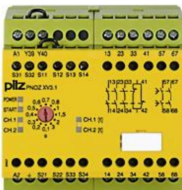
Safety relay (standalone) Inputs: 1-/2-channel wiring with/without detection of shorts across contacts Outputs: 3 N/O, 1 N/C, 2 N/O delayed UB 24-240 V AC/DC, width: 90 mm, integral screw terminals, Monitoring E-STOP, safety gates with 2 delay-on de-energisation contacts. Release time 12 stages from 0 - 3 s.
