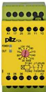
Safety relay (standalone) Inputs: Single-channel wiring Outputs: 1 N/O, 2 N/C UB 230 V AC, width: 45 mm, integral screw terminals, delay-on energisation pulse timer, pulse times 12 stages from 0 - 300 s.
