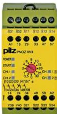
Safety relay (standalone) Inputs: 1-/2-channel wiring with/without detection of shorts across contacts Outputs: 3 N/O, 2 N/O delayed UB 24 V DC, width: 45 mm, integral screw terminals, Monitoring E-STOP, safety gates with 2 delay-on de-energisation contacts. Release time 12 stages from 0 - 30 s.
