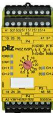
Safety relay (standalone) Inputs: 1-/2-channel wiring with/without detection of shorts across contacts Outputs: 3 N/O, 2 N/O (t = 0 - 30 s). Automatic/monitored start UB 24 V DC, width: 45 mm, plug-in terminals of screw type Monitoring E-STOP, safety gates.
