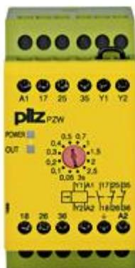
Safety relay (standalone) Inputs: Single-channel wiring Outputs: 1 N/O, 2 N/C UB 110-120 V AC, width: 45 mm, integral screw terminals Pulse timer, pulse times 12 stages from 0 - 3 s.
