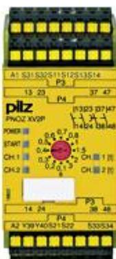
Safety relay (standalone) Inputs: 1-/2-channel wiring with/without detection of shorts across contacts Outputs: 2 N/O, 2 N/O (t = 0 - 3 s) . Automatic/monitored start UB 24 V DC, width: 45 mm, plug-in spring-loaded terminals. Monitoring E-STOP, safety gates.
