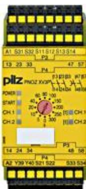
Safety relay (standalone) Inputs: 1-/2-channel wiring with/without detection of shorts across contacts Outputs: 3 N/O, 2 N/O (t = 0 - 300 s). Automatic/monitored start UB 24 V DC, width: 45 mm, plug-in spring-loaded terminals. Monitoring E-STOP, safety gates.
