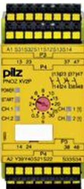
Safety relay (standalone) Inputs: 1-/2-channel wiring with/without detection of shorts across contacts Outputs: 2 N/O, 2 N/O (t = 0 - 30 s). Automatic/monitored start UB 24 V DC, width: 45 mm, plug-in spring-loaded terminals. Monitoring E-STOP, safety gates.
