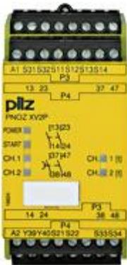
Safety relay (standalone) Inputs: 1-/2-channel wiring with/without detection of shorts across contacts Outputs: 2 N/O, 2 N/O (t = 0.5 s fixed). Automatic/monitored start UB 24 V DC, width: 45 mm, plug-in terminals of screw type Monitoring E-STOP, safety gates.
