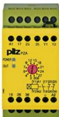
Safety relay (standalone) Inputs: Single-channel wiring Outputs: 1 N/O, 2 N/C UB 110-120 V AC, width: 45 mm, integral screw terminals, delay-on energisation pulse timer, pulse times 12 stages from 0 - 30 s.
