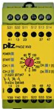
Safety relay (standalone) Inputs: 1- / 2-channel wiring with detection of shorts across contacts Outputs: 2 N/O, 2 N/O delayed UB 24 V DC, width: 90 mm, integral screw terminals, Monitoring E-STOP, safety gates with 2 delay-on de-energisation contacts. Release time 12 stages from 0 - 300 s.
