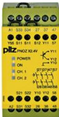
Safety relay (standalone) Inputs: 1-/2-channel wiring with/without detection of shorts across contacts Outputs: 4 N/O delayed, 1 semiconductor instantaneous UB 24 V DC, width: 45 mm, integral screw terminals, Monitoring E-STOP, safety gates with 4 delay-on de-energisation contacts. Release time 1 s fixed and retriggerable.
