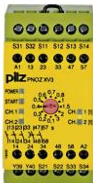
Safety relay (standalone) Inputs: 1-/2-channel wiring with/without detection of shorts across contacts Outputs: 3 N/O, 2 N/O delayed UB 24 V DC, width: 45 mm, integral screw terminals, Monitoring E-STOP, safety gates with 2 delay-on de-energisation contacts. Release time 12 stages from 0 - 3 s.
