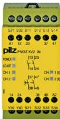
Safety relay (standalone) Inputs: 1- / 2-channel wiring with detection of shorts across contacts Outputs: 2 N/O, 2 N/O delayed UB 24 V DC, width: 45 mm, integral screw terminals, Monitoring E-STOP, safety gates with 2 delay-on de-energisation contacts. Release time 3 s fixed.
