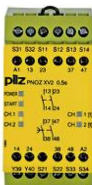
Safety relay (standalone) Inputs: 1- / 2-channel wiring with detection of shorts across contacts Outputs: 2 N/O, 2 N/O delayed UB 24 V DC, width: 45 mm, integral screw terminals, Monitoring E-STOP, safety gates with 2 delay-on de-energisation contacts. Release time 0.5 s fixed.
