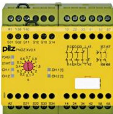
Safety relay (standalone) Inputs: 1-/2-channel wiring with/without detection of shorts across contacts Outputs: 3 N/O, 1 N/C, 2 N/O delayed UB 24 V DC, width: 90 mm, integral screw terminals, Monitoring E-STOP, safety gates with 2 delay-on de-energisation contacts. Release time 12 stages from 0 - 3 s.
