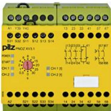
Safety relay (standalone) Inputs: 1-/2-channel wiring with/without detection of shorts across contacts Outputs: 3 N/O, 1 N/C, 2 N/O delayed UB 24 V DC, width: 90 mm, integral screw terminals, Monitoring E-STOP, safety gates with 2 delay-on de-energisation contacts. Release time 12 stages from 0 - 30 s.
