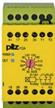
Safety relay (standalone) Inputs: Single-channel wiring Outputs: 1 N/O, 2 N/C UB 110 - 120 V AC, width: 45 mm, integral screw terminals, delay-on energisation pulse timer, pulse times 12 stages from 0 - 300s.
