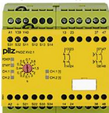
Safety relay (standalone) Inputs: 1-/2-channel wiring with/without detection of shorts across contacts Outputs: 2 N/O, 2 N/O delayed UB 24-240 V AC/DC, width: 90 mm, integral screw terminals, Monitoring E-STOP, safety gates with 2 delay-on de-energisation contacts. Release time 12 stages from 0 - 3 s.
