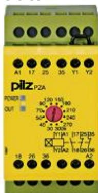
Safety relay (standalone) Inputs: Single-channel wiring Outputs: 1 N/O, 2 N/C UB 24 V DC, width: 45 mm, integral screw terminals, delay-on energisation pulse timer, pulse times 12 stages from 0 - 300 s.
