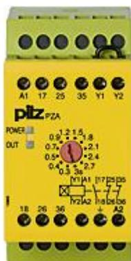
Safety relay (standalone) Inputs: Single-channel wiring Outputs: 1 N/O, 2 N/C UB 230 V AC, width: 45 mm, integral screw terminals, delay-on energisation pulse timer, pulse times 12 stages from 0 - 3 s.
