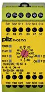
Safety relay (standalone) Inputs: 1-/2-channel wiring with/without detection of shorts across contacts Outputs: 3 N/O, 2 N/O delayed UB 24 V DC, width: 45 mm, integral screw terminals, Monitoring E-STOP, safety gates with 2 delay-on de-energisation contacts. Release time 12 stages from 0 - 300 s.
