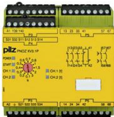
Safety relay (standalone) Inputs: 1-/2-channel wiring with/without detection of shorts across contacts Outputs: 3 N/O, 1 N/C, 2 N/O (t = 0 - 30 s). Automatic/monitored start UB 24 - 240 V AC/DC, width: 90 mm, plug-in terminals of screw type Monitoring E-STOP, safety gates.
