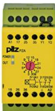
Safety relay (standalone) Inputs: Single-channel wiring Outputs: 1 N/O, 2 N/C. UB 230 V AC, width: 45 mm, integral screw terminals, delay-on energisation pulse timer, pulse times 12 stages from 0 - 30 s.
