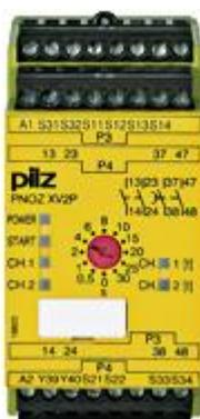
Safety relay (standalone) Inputs: 1-/2-channel wiring with/without detection of shorts across contacts Outputs: 2 N/O, 2 N/O (t = 0 - 30 s). Automatic/monitored start UB 24 V DC, width: 45 mm, plug-in terminals of screw type Monitoring E-STOP, safety gates.
