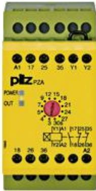
Safety relay (standalone) Inputs: Single-channel wiring Outputs: 1 N/O, 2 N/C UB 24 V DC, width: 45 mm, integral screw terminals, delay-on energisation pulse timer, pulse times 12 stages from 0 - 30 s.
