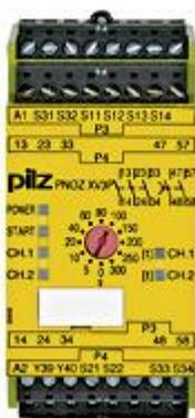
Safety relay (standalone) Inputs: 1-/2-channel wiring with/without detection of shorts across contacts Outputs: 3 N/O, 2 N/O (t = 0 - 300 s). Automatic/monitored start UB 24 V DC, width: 45 mm, plug-in terminals of screw type Monitoring E-STOP, safety gates.
