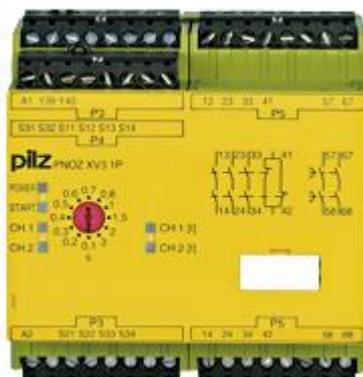
Safety relay (standalone) Inputs: 1-/2-channel wiring with/without detection of shorts across contacts Outputs: 3 N/O, 1 N/C, 2 N/O (t = 0 - 300 s). Automatic/monitored start UB 24 V DC, width: 90 mm, plug-in terminals of screw type Monitoring E-STOP, safety gates.
