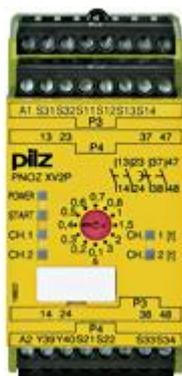
Safety relay (standalone) Inputs: 1-/2-channel wiring with/without detection of shorts across contacts Outputs: 2 N/O, 2 N/O (t = 0 - 3 s) . Automatic/monitored start UB 24 V DC, width: 45 mm, plug-in terminals of screw type Monitoring E-STOP, safety gates.
