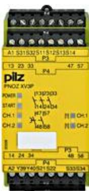
Safety relay (standalone) Inputs: 1-/2-channel wiring with/without detection of shorts across contacts Outputs: 3 N/O, 2 N/O (t = 0.5 s fixed). Automatic/monitored start UB 24 V DC, width: 45 mm, plug-in terminals of screw type Monitoring E-STOP, safety gates.
