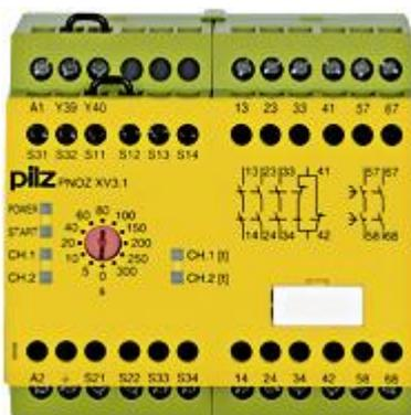
Safety relay (standalone) Inputs: 1-/2-channel wiring with/without detection of shorts across contacts Outputs: 3 N/O, 1 N/C, 2 N/O delayed UB 24 V DC, width: 90 mm, integral screw terminals, Monitoring E-STOP, safety gates with 2 delay-on de-energisation contacts. Release time 12 stages from 0 - 300 s.
