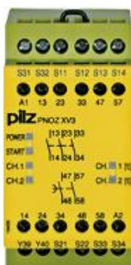
Safety relay (standalone) Inputs: 1-/2-channel wiring with/without detection of shorts across contacts Outputs: 3 N/O, 2 N/O delayed UB 24 V DC, width: 45 mm, integral screw terminals, Monitoring E-STOP, safety gates with 2 delay-on de-energisation contacts. Release time 0.5 s fixed.
