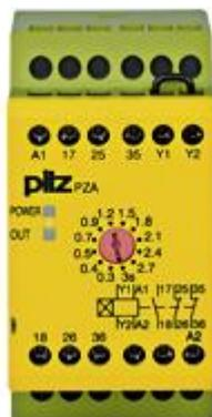
Safety relay (standalone) Inputs: Single-channel wiring Outputs: 1 N/O, 2 N/C UB 24 V DC, width: 45 mm, integral screw terminals, delay-on energisation pulse timer, pulse times 12 stages from 0 - 3 s.
