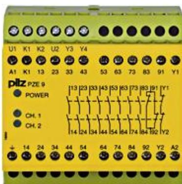
Contact expansion Inputs: ability to detect shorts across contacts Outputs: 8 N/O, 1 N/C UB 230 - 240 V AC, width: 90 mm, Contact block for contact expansion + amplification in connection with safety-related control components.
