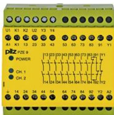
Contact expansion Inputs: ability to detect shorts across contacts Outputs: 8 N/O, 1 N/C UB 42 V AC, width: 90 mm, Contact block for contact expansion + amplification in connection with safety-related control components.
