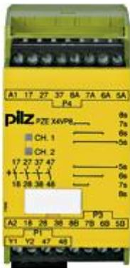
Contact expansion Inputs: Single-channel wiring Outputs: 4 N/O (t = 5, 6, 7, 8 s fixed). UB 24 V DC, width: 45 mm, plug-in terminals of screw type. Contact block for contact expansion in connection with safety-related control components.
