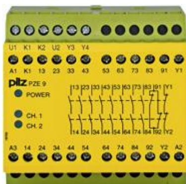
Contact expansion Inputs: ability to detect shorts across contacts Outputs: 8 N/O, 1 N/C UB 24 V DC, width: 90 mm, Contact block for contact expansion + amplification in connection with safety-related control components.
