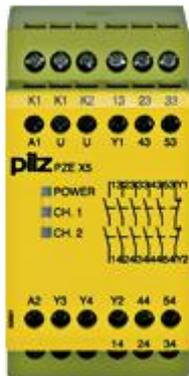
Contact expansion Inputs: 1-/2-channel wiring with/without detection of shorts across contacts Outputs: 5 N/O UB 24 V DC, width:45 mm, integral screw terminals, Contact block for contact expansion in connection with safety-related control components.
