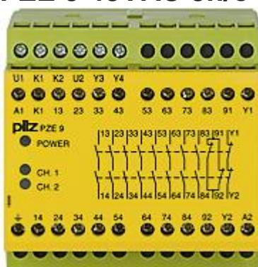
Contact expansion Inputs: ability to detect shorts across contacts Outputs: 8 N/O, 1 N/C UB 48 V AC, width: 90 mm, Contact block for contact expansion + amplification in connection with safety-related control components.
