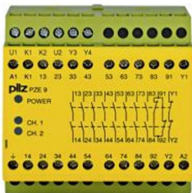
Contact expansion Inputs: ability to detect shorts across contacts Outputs: 8 N/O, 1 N/C UB 110 - 120 V AC, width: 90 mm, Contact block for contact expansion + amplification in connection with safety-related control components.
