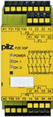
Contact expansion Inputs: 1-/2-channel wiring with/without detection of shorts across contacts Outputs: 8 N/O, 1 N/C. UB 24 V AC/DC, width: 90 mm, plug-in spring-loaded terminals.
