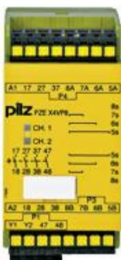
Contact expansion Inputs: Single-channel wiring Outputs: 4 N/O (t = 5, 6, 7, 8 s fixed). UB 24 V DC, width: 45 mm, plug-in spring-loaded terminals. Contact block for contact contact expansion in connection with safety-related control components.
