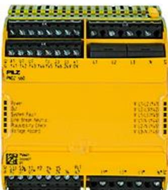
PNOZsigma voltage monitoring relay for applications up to PLe acc. EN ISO 13849-1 and SIL cl 3 acc. EN IEC 62061, UB = 100-240VACDC, Outputs: 3 n/o, 1 n/c, 6 so, width: 90mm, plug-in terminals of screw type, expandable with PNOZsigma contact expansions?
