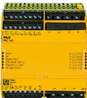
PNOZsigma voltage monitoring relay for applications up to PLe acc. EN ISO 13849-1 and SIL cl 3 acc. EN IEC 62061, UB = 24-48VACDC, Outputs: 3 n/o, 1 n/c, 6 so, width: 90mm, plug-in terminals of screw type, expandable with PNOZsigma contact expansions?
