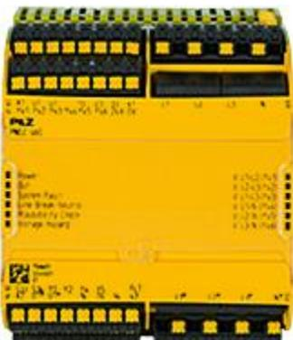
PNOZsigma voltage monitoring relay for applications up to PLe acc. EN ISO 13849-1 and SIL cl 3 acc. EN IEC 62061, UB = 100-240VACDC, Outputs: 3 n/o, 1 n/c, 6 so, width: 90mm, plug-in spring-loaded terminals, expandable with PNOZsigma contact expansions.
