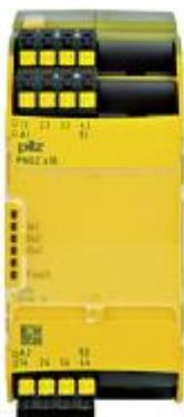
PNOZsigma Contact expansion. Outputs: 4 N/O, 1 N/C. UB 24 V DC, 12A DC1 switching load, width: 45 mm, plug-in spring-loaded terminals. Contact block for contact expansion in connection with safety-related control components.
