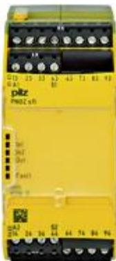
PNOZsigma Contact expansion. Outputs: 8 N/O, 1 N/C UB 24 V DC, width: 45 mm, plug-in terminals of screw type
