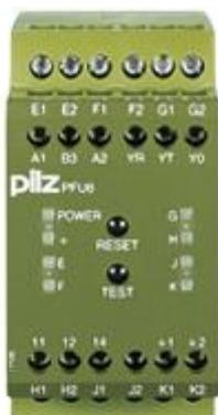
Fault voltage monitoring of welding transformers in accordance with V DE 0545; 6 Measuring input circuits 0 - 690 V AC/DC; 50 Hz-1 kHz; Response value 24 V AC/DC; Width: 45 mm; UB 24 - 240 V AC/DC.
